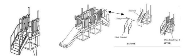
Drill 3/8" holes through posts, slide guards, and protrusions of roof that are inserted into tops of posts. Attach slide guards and roof with hardware provided.
