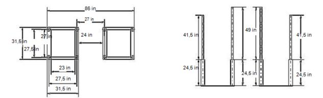
Situate main frames so that the longer posts face inside and the shorter posts are outside. Stack components over the posts as shown below.
