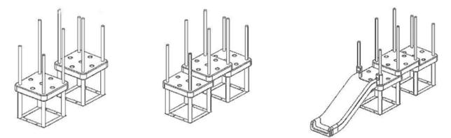
Align panels 1 and panel 2, hold them together, then slide them over the posts. On the opposite side, align panels 1 with the panel 2 and slide them over the posts together.
