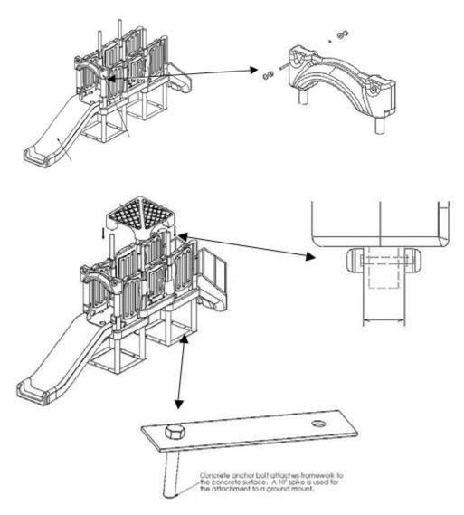
Secure main structure to solid surface using anchor bolts, or secure structure to ground using 0,47 x 0,98in spikes. (Not provided)
